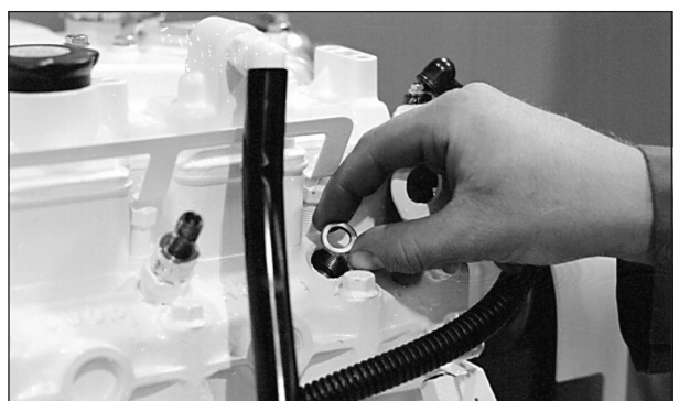
Figure 17: Remove and replace copper sealing washer.
