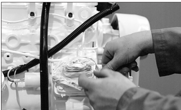
Figure 13: Cover lines, inlets and injection pump outlets.
